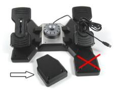
First remove the heel plates if fitted, you won't be using these as the screw holes they fit into will have screws in them.
