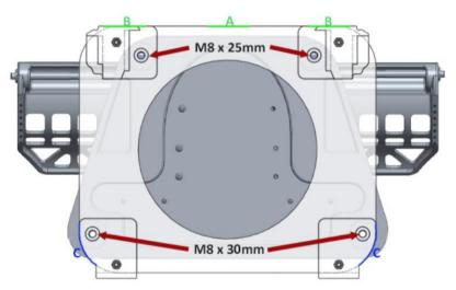
For ease of mounting, sit the TPR Pedals on their back to gain access to the base.
