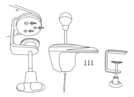
Fitting the QRPro Thrustmaster TH8A Gearstick Quick Release Plate Kit
