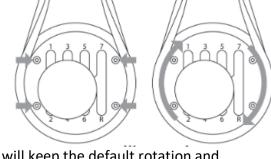
the rig towards the front and therefore we will keep the default rotation and orientation of the TH8A as it comes out of the box as shown here.
